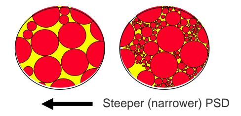
PSD Steepness is a measure of the range of particle sizes included in a mineral product:
